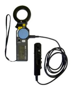
This is new measuring method for AC leakage current for single phase power system.
